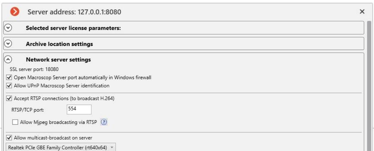
To make a RTSP connection it is possible to use TCP (RTSP over TCP) **or** HTTP (RTSP over HTTP) connections. UDP connections (RTSP over UDP) are not supported.
