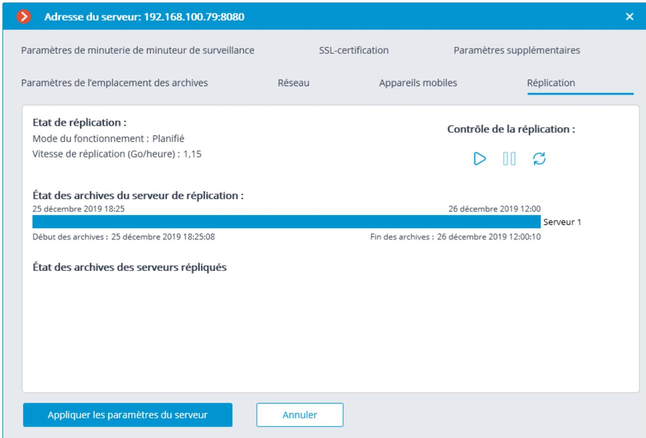
The screenshot displays the configuration interface for the Eocortex application, specifically the replication settings for a server. The window title is "Adresse du serveur: 192.168.100.79:8080". The interface is divided into several tabs: "Paramètres de minuterie de minuteur de surveillance", "SSL-certification", "Paramètres supplémentaires", "Paramètres de l'emplacement des archives", "Réseau", "Appareils mobiles", and "Réplication". The "Réplication" tab is currently selected.
