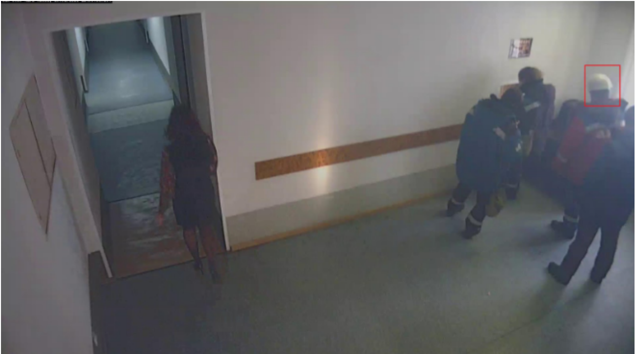
Insufficient contrast, badly distinguishable boundaries of objects, flaring, image compression too high.
